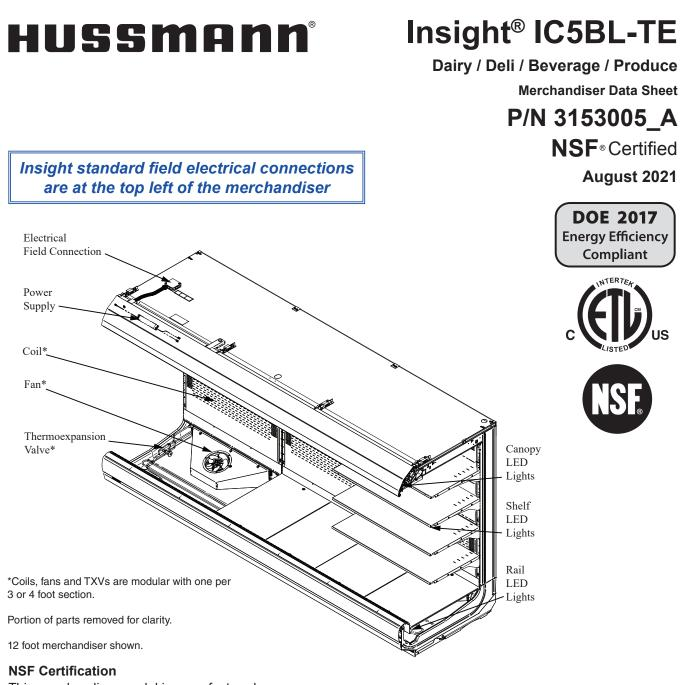
This merchandiser model is manufactured to meet NSF/ANSI (National Sanitation Foundation) Standard #7 requirements for construction, materials and cleanability.
