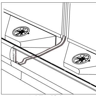
Apply Neutral Curing Silicone Sealant
