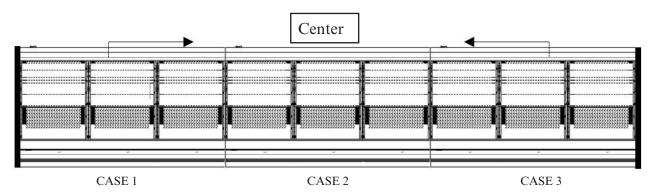
2. Place fascia trim along fascia surface adjacent to ends to eliminate gaps at the ends of the lineup.
