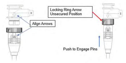
**C.** Turn locking ring until all three arrows are aligned.
