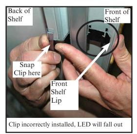
Shelf LED clips must be first inserted into the front lip underneath the shelf as shown at left. Next the retaining clip is "snapped on" to the rear of the LED clip.
