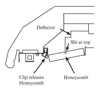
Damaged honeycomb must be replaced.
