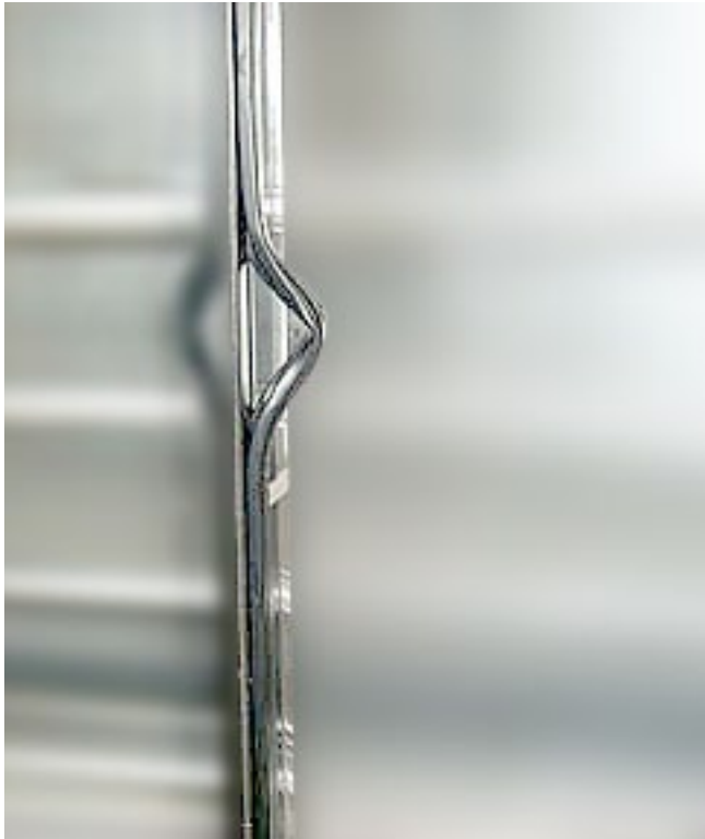
Improperly Installed or Damaged Gasket
