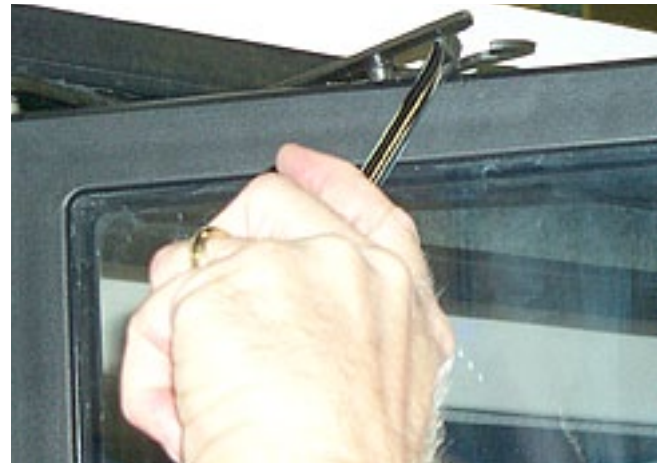
Lift Door Retainer Over Shoulder Screw
