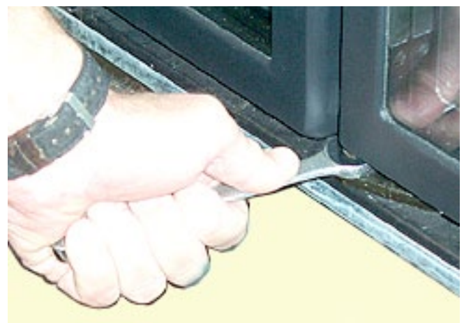
Adjust Closing Torque
