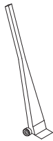
Lever Bar (also know as a Mule, Johnson Bar, J-bar, Lever Dolly or pry lever)
