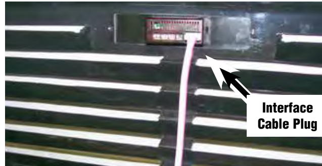
Unplug Safe-NET III Interface Cable
