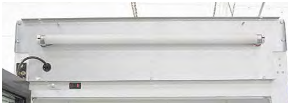
Display Cover Panel Removed
