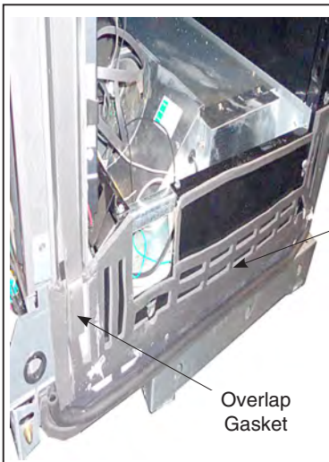
Figure 5B, Part 2. Apply Gaskets to Right End of RL/RM/RMF and RLN/RMN
