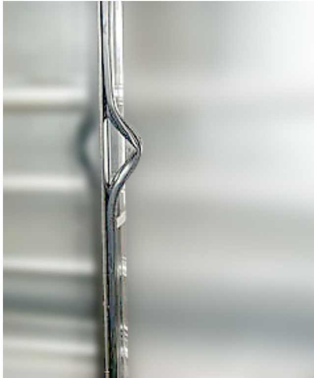
Improperly Installed or Damaged Gasket
